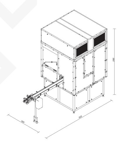
Cup filling and sealing machine **RFS 120** is designed for yogurt, sour cream, kefir to be filled into pre-made containers with aluminum foil and/or lids. Rotary type machine has 3 rows.
