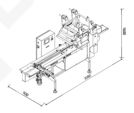
**PM** is a horizontal Flow-Pack type machine. Packs are sealed on three sides from a roll of heatsealable packaging film. It is compatible with AR2T curd filling and wrapping machine.
