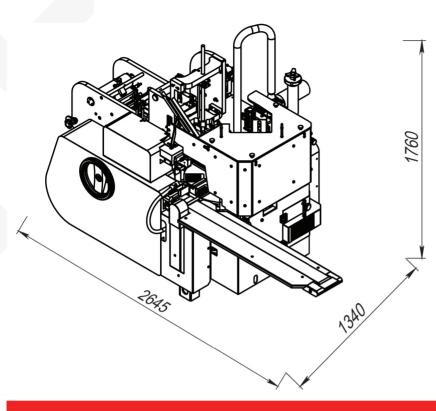
Ice cream filling and wrapping machine **ARG** is for sandwich ice-cream packaging with or without waffles to bricks.
