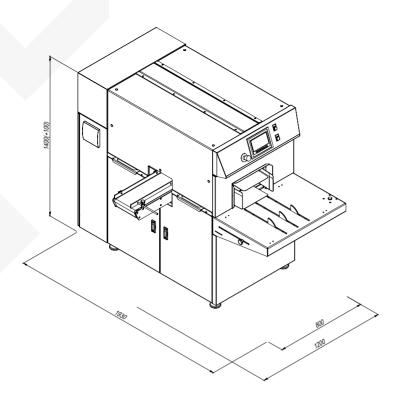
**DSU** is a semi-automatic cartoning machine used for grouping and stacking of butter bricks. Bricks are packed by ARM or any other filling and wrapping machine. It serves as an exceptionally reliable and cost-effective end of the line solution. Case packer operates at capacity of up to 100 bricks per minute. Different box sizes are possible.
