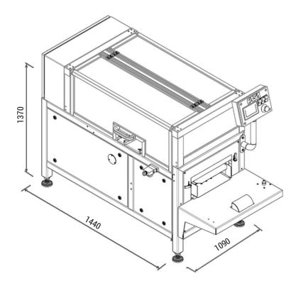
**DSU** is a semi-automatic cartoning machine used for grouping and stacking of butter bricks packed with ARM or other filling and wrapping machines. It serves as exceptionally reliable and cost-effective end of the line solution.
